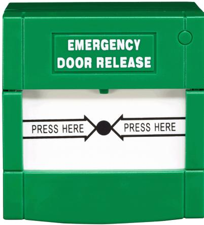
The Call Point can be activated without power supply in emergencies. It is typically located on fire escape doors. The main function is to override the electrical locking devices in case of emergency. Using the provided key to reset the switch.
